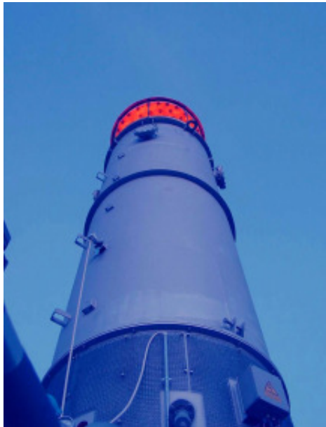
One of the two flares burning the residual gas out of the gas quality standard
